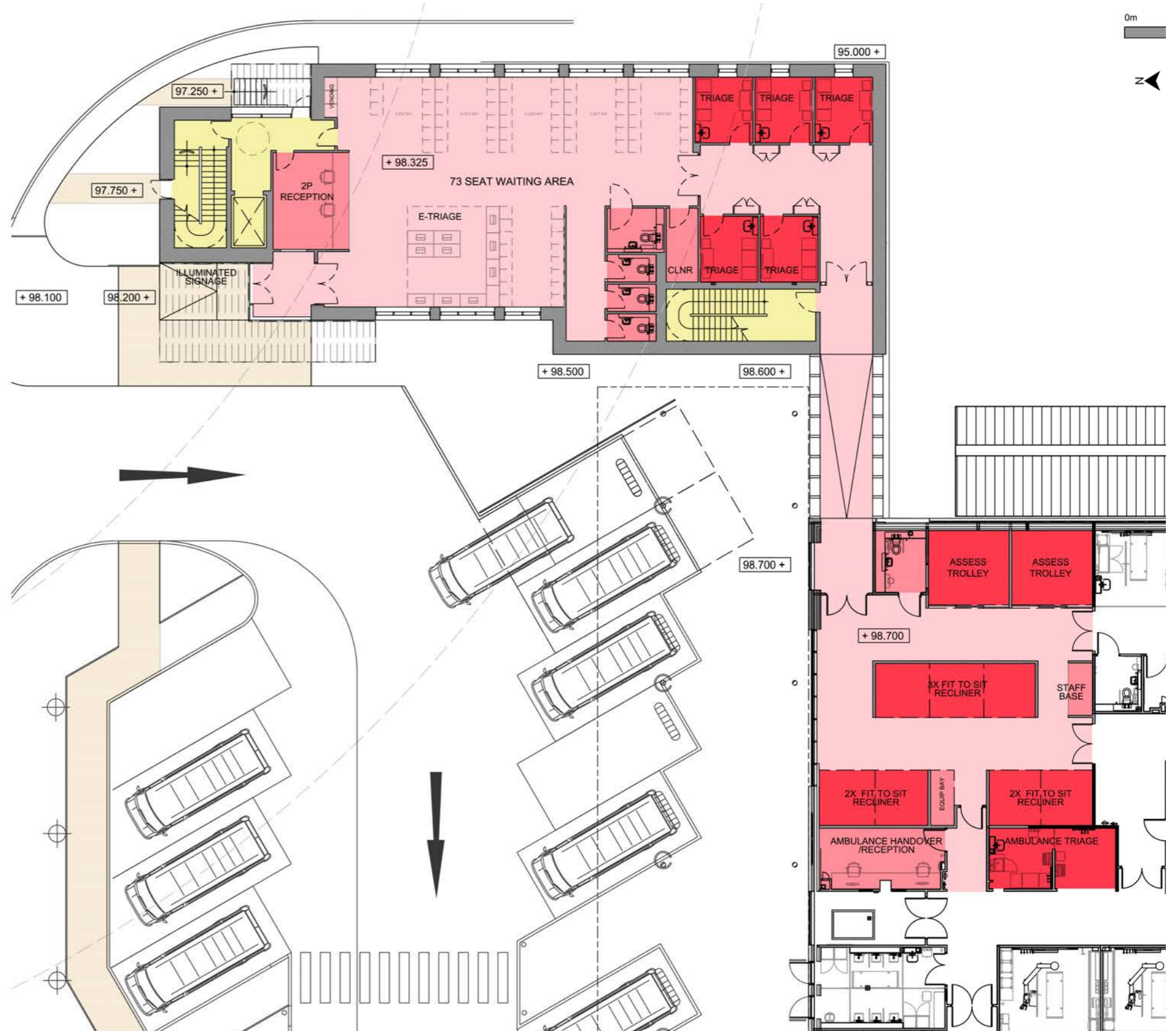
Stage 01 L01 layout with entrance on the northwestern corner of the building, reception remote from triage area
